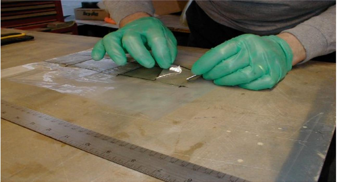
Once the cloth is in place use your razor blade to remove the remaining layer of plastic from the fiberglass cloth.
