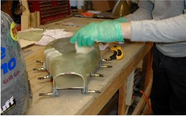
Now cut a few strips of the peel-ply that are large enough to cover the glass you just applied to your work and place them on top of your glass using the foam rubber to tamp them down.
