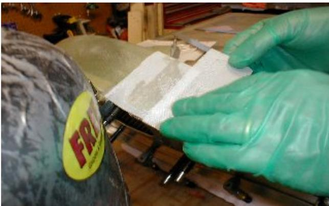
The extra resin from the cloth will be absorbed into the peel-ply and will hold it in place for later removal.
