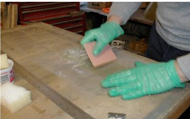
Next use the squeegee to work all the extra resin away from the cloth so that only the minimum amount of resin is in the cloth. Just work it off to the side until it's sitting in a blob in the drop cloth away from the fiberglass cloth.
