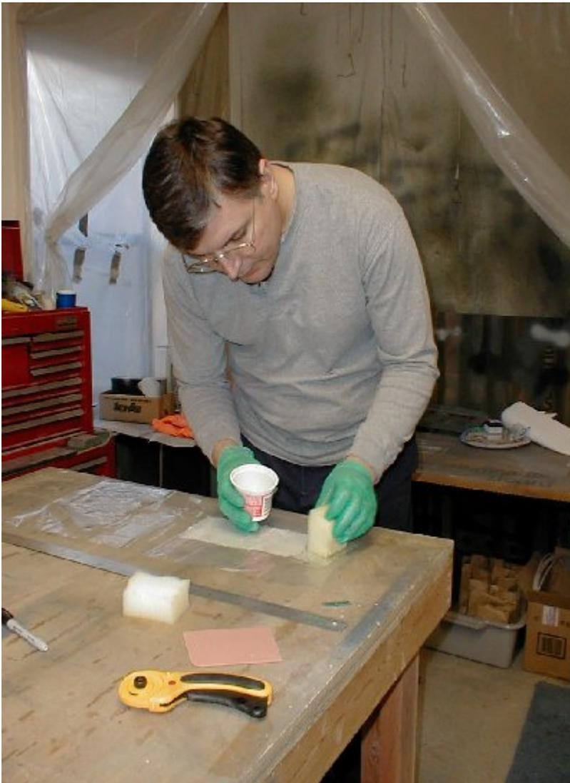
Use one of your two inch foam rubber sponges to dip in the resin and dab this on the cloth until it's completely saturated with the resin. The fiberglass cloth should actually start turning clear when it's saturated with resin.
